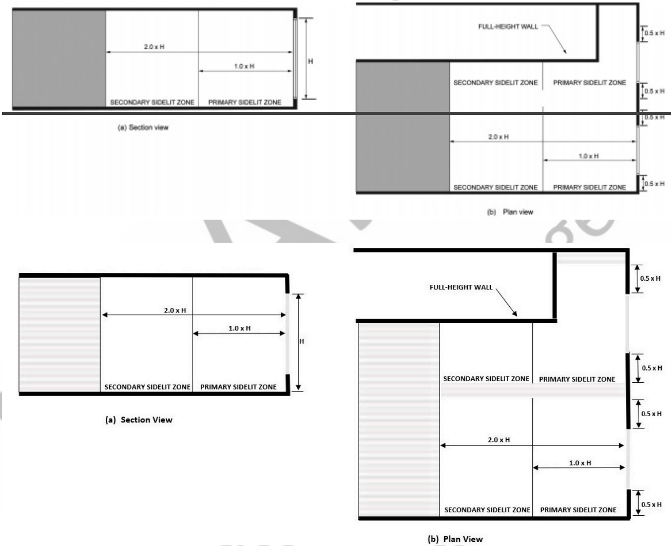
FIGURE C405.2.4.2(1) PRIMARY AND SECONDARY SIDELIT DAYLIGHT ZONES
