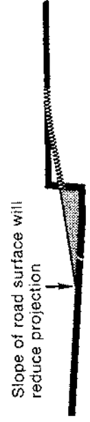
Curb ramp partially recessed in sidewalk
