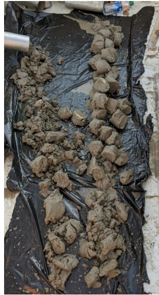
Figure 7. Vibracore extruded on deck for chemical sampling
