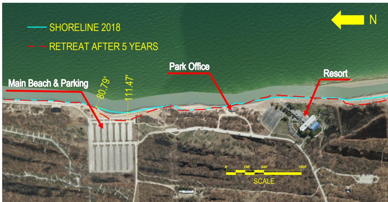
Figure C-17: 5-year shoreline projection without mitigation, Area 3 (map data: Google, USDA Farm Service Agency)
