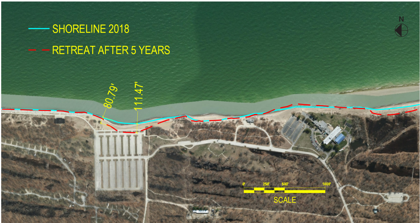
Figure 34: 5-year shoreline projection without mitigation, Area 3 (map data: Google, USDA Farm Service Agency)
