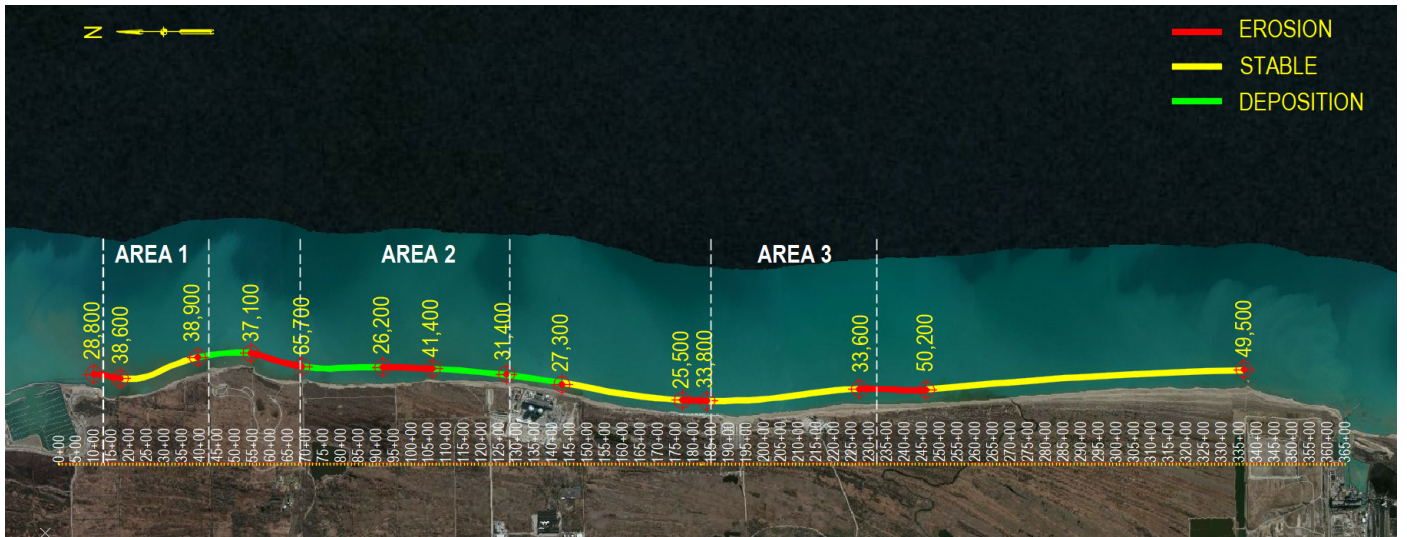
Figure 39: Potential net longshore sediment transport rates (in yd³/year) for the IBSP after installation of stabilization structures (map data: Google, USDA Farm Service Agency)
