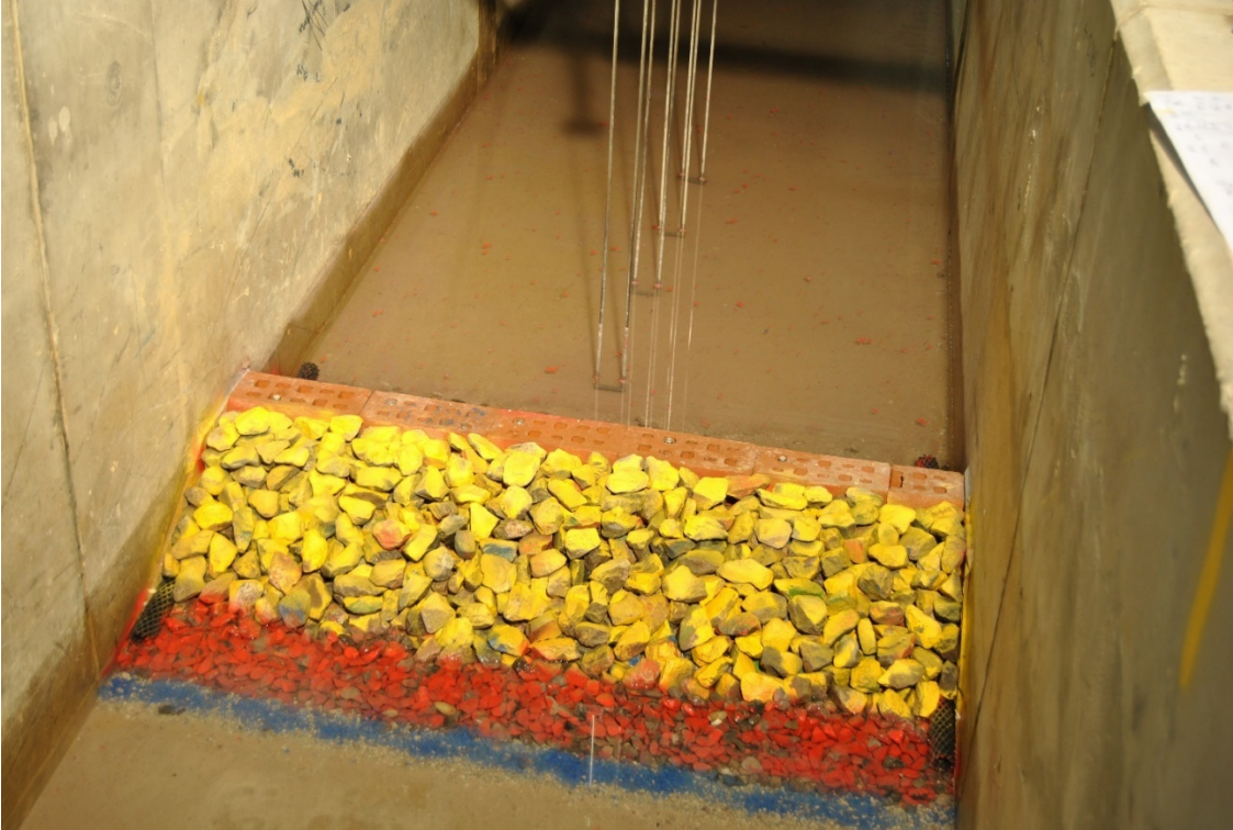
Figure 6.12: 3-6 tonne rock armour structure – pre-test photograph
