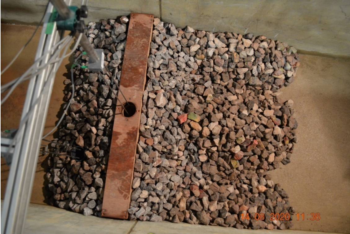
Figure 2.3: Example transmission test structure with impermeable (plywood) crest
