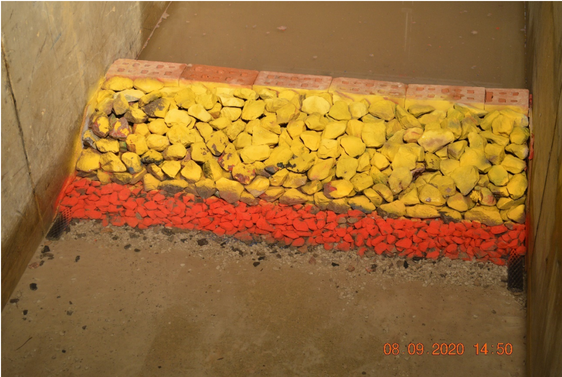
Figure 6.7: 6-9 tonne rock armour structure – pre-test photograph
