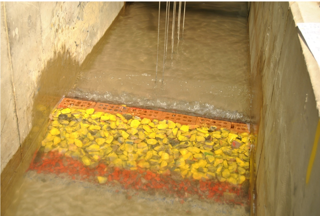
Figure 6.15: 3-6 tonne rock armour structure – post Test Part 03 photograph (WC_EXT_WL_01)
