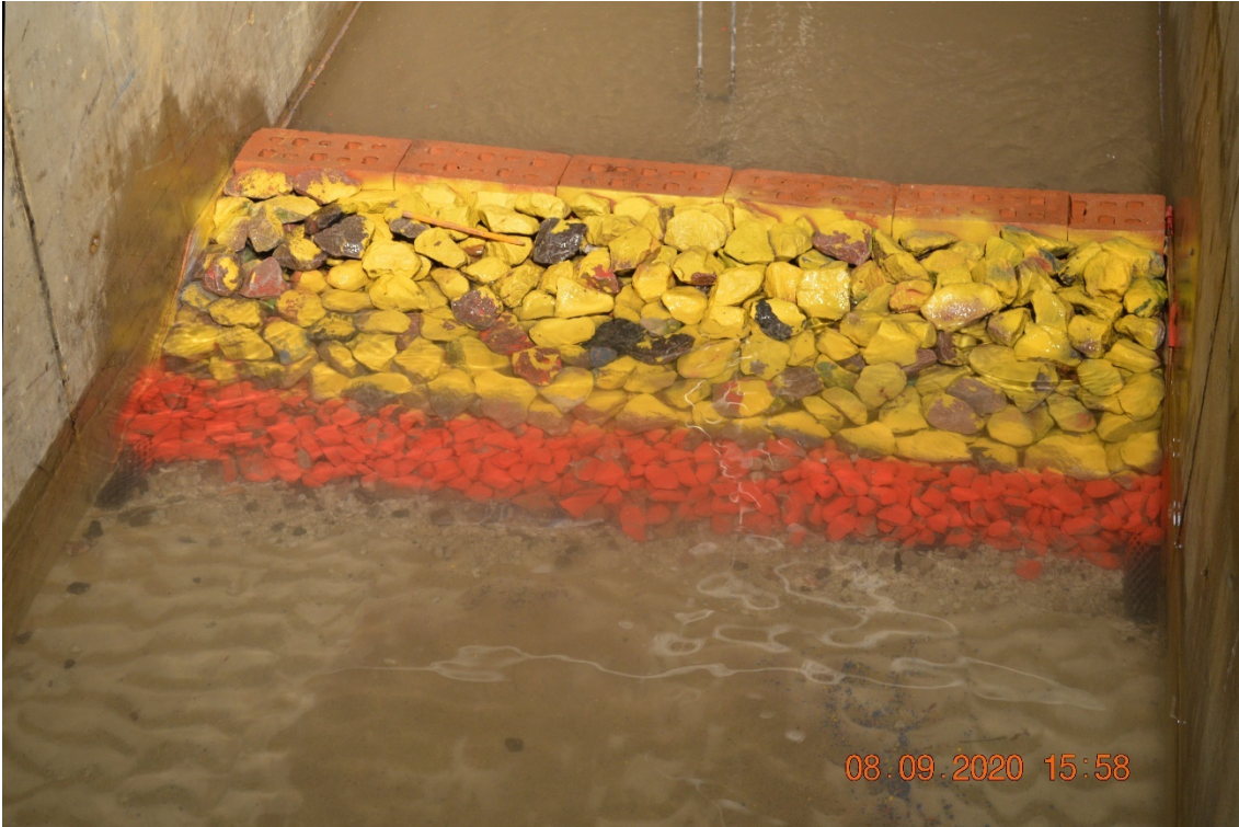
Figure 6.9: 6-9 tonne rock armour structure – post Test Part 02 photograph (WC_HIGH_WL)
