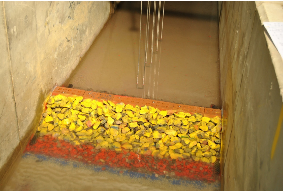
Figure 6.13: 3-6 tonne rock armour structure – post Test Part 01 photograph (WC_LOW_WL)
