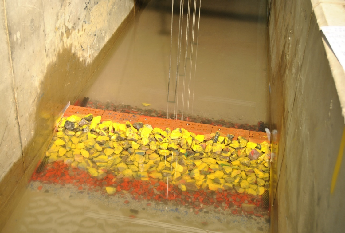
Figure 6.16: 3-6 tonne rock armour structure – post Test Part 04 photograph (WC_EXT_WL_02)
