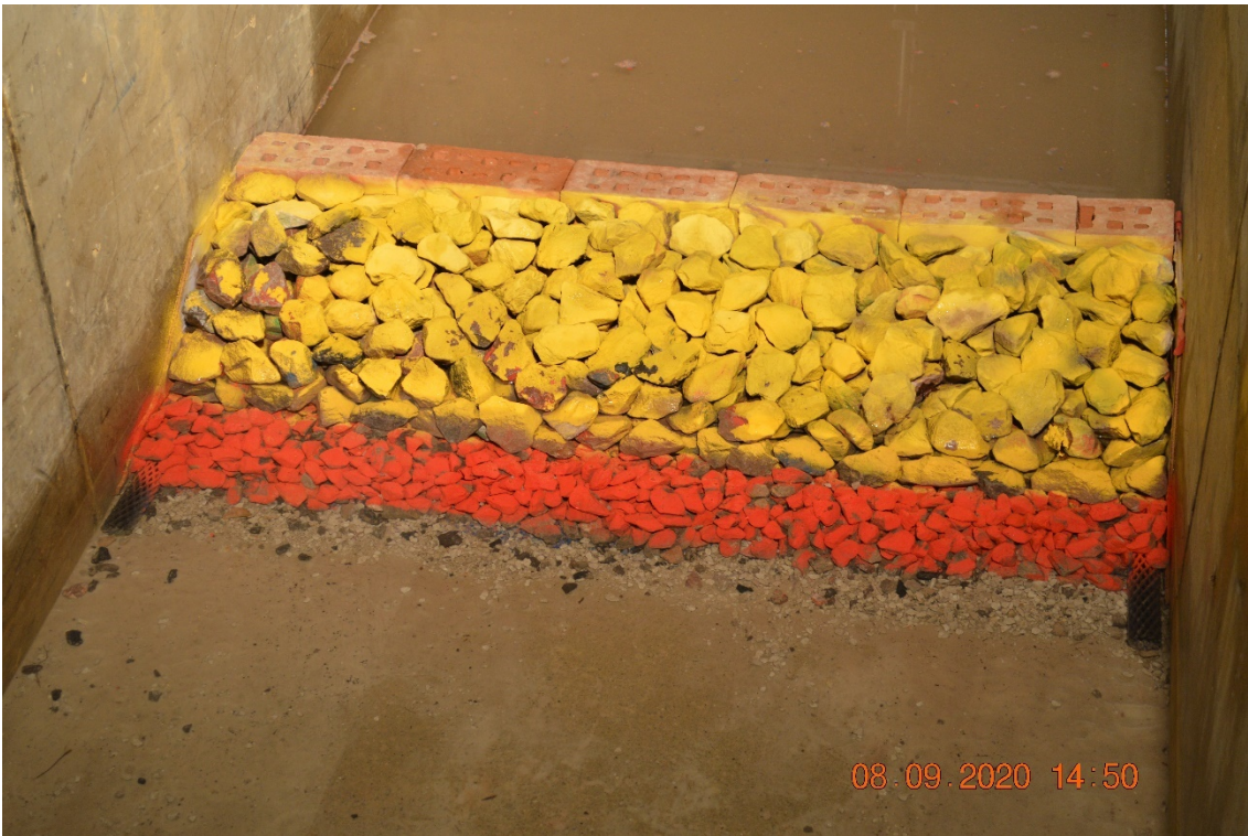
Figure 6.8: 6-9 tonne rock armour structure – post Test Part 01 photograph (WC_LOW_WL)
