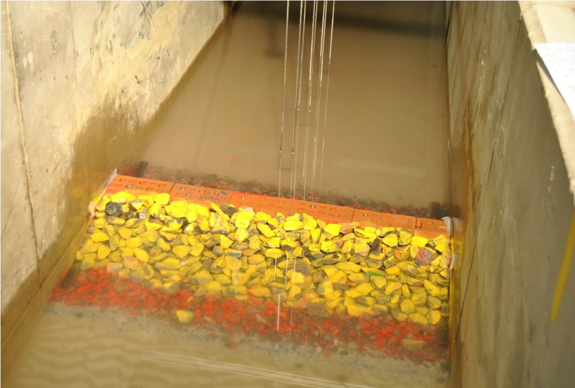
Figure 6.14: 3-6 tonne rock armour structure – post Test Part 02 photograph (WC_HIGH_WL)
