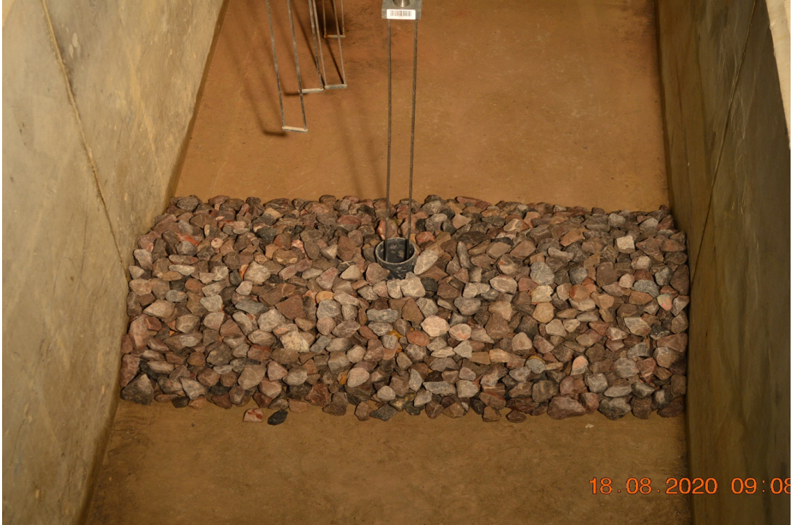
Figure 2.11: Photograph of Structure_15 in flume prior to testing
