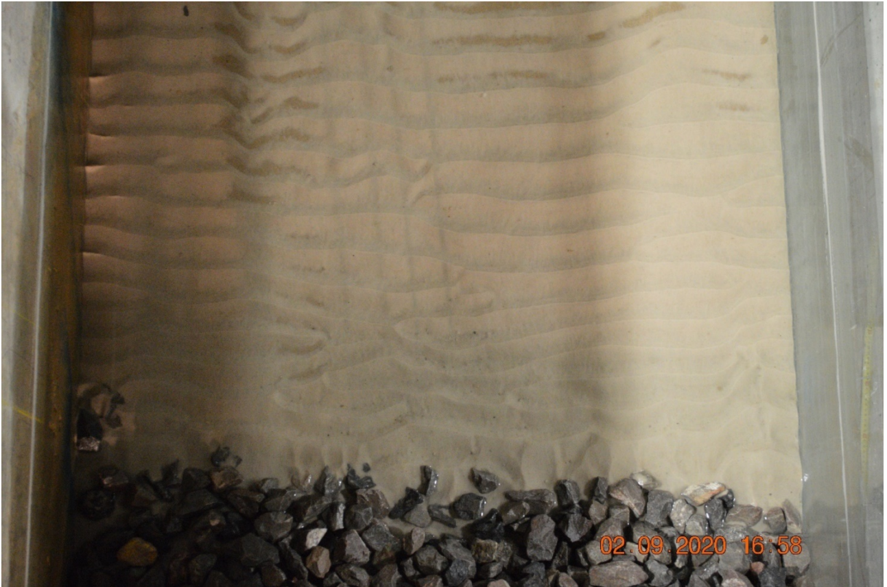
Figure B.5: Healthy Port Futures sand retention post-test photograph (Leeward of final structure)
