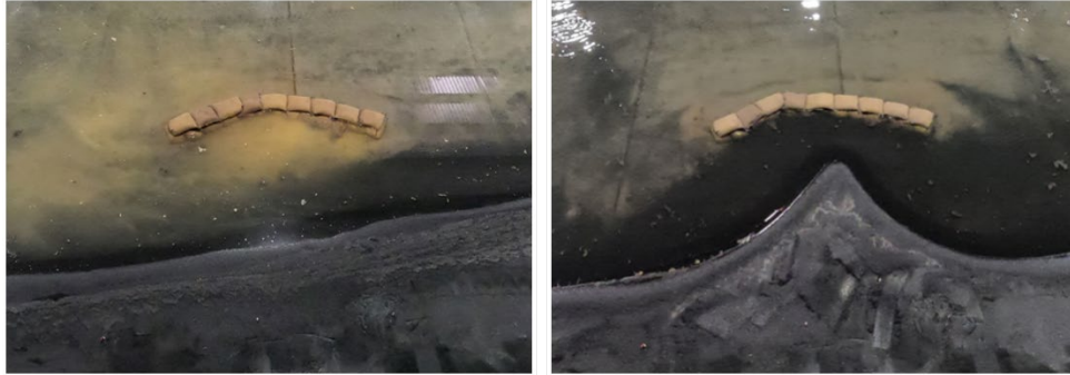
Figure 6: Example of a Tombolo Forming During the Laboratory Tests
