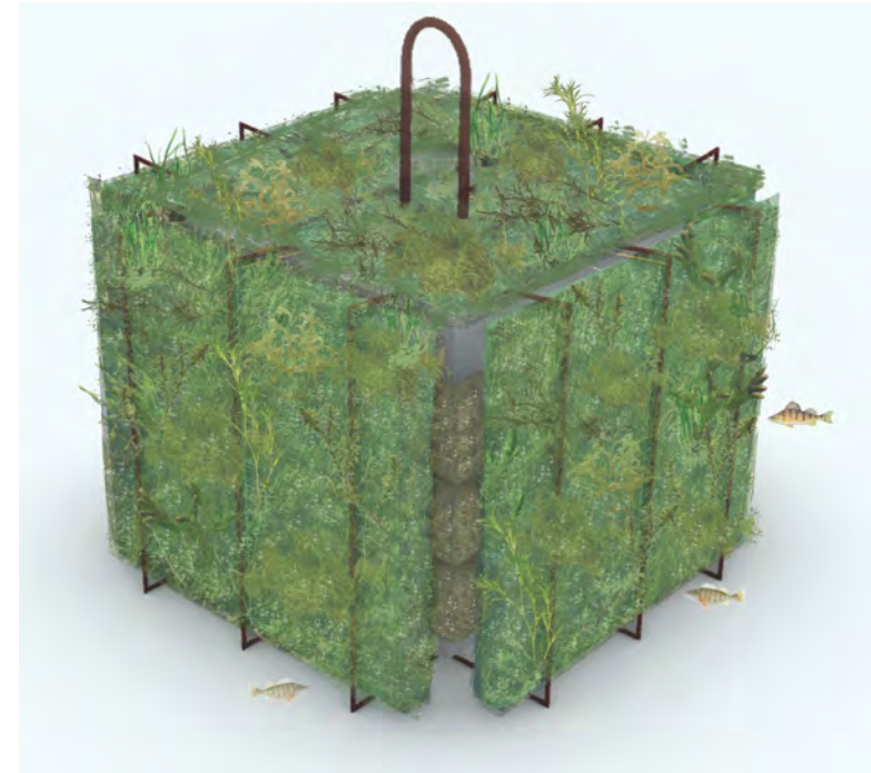
VEGETATED CONCRETE BLOCK - AXONOMETRIC
